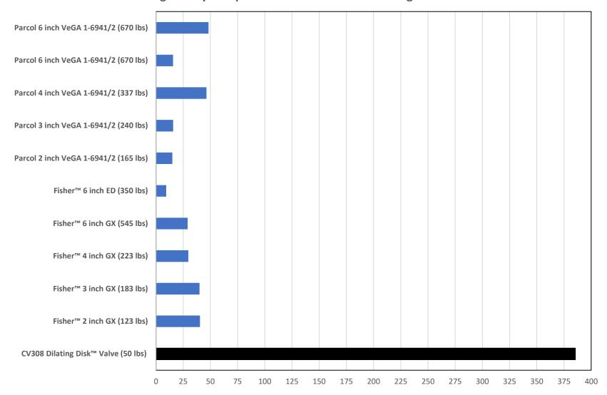
Rangeability - Maximum C<sub>v</sub> (Full Open) over Minimum C<sub>v</sub> (10% of Full Open)
