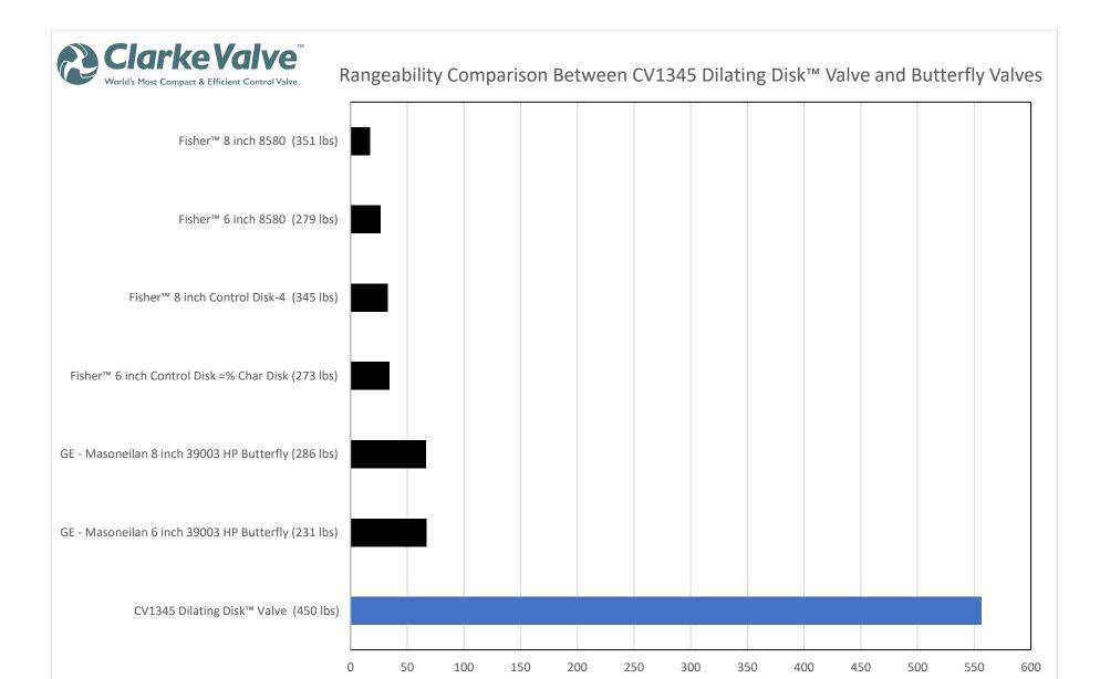
Rangeability - Maximum C<sub>V</sub> (Full Open) over Minimum C<sub>V</sub> (10% of Full Open)
